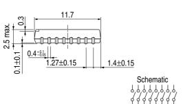
Unless otherwise specified, tolerance :  $\pm 0.3$  (Unit : mm)
